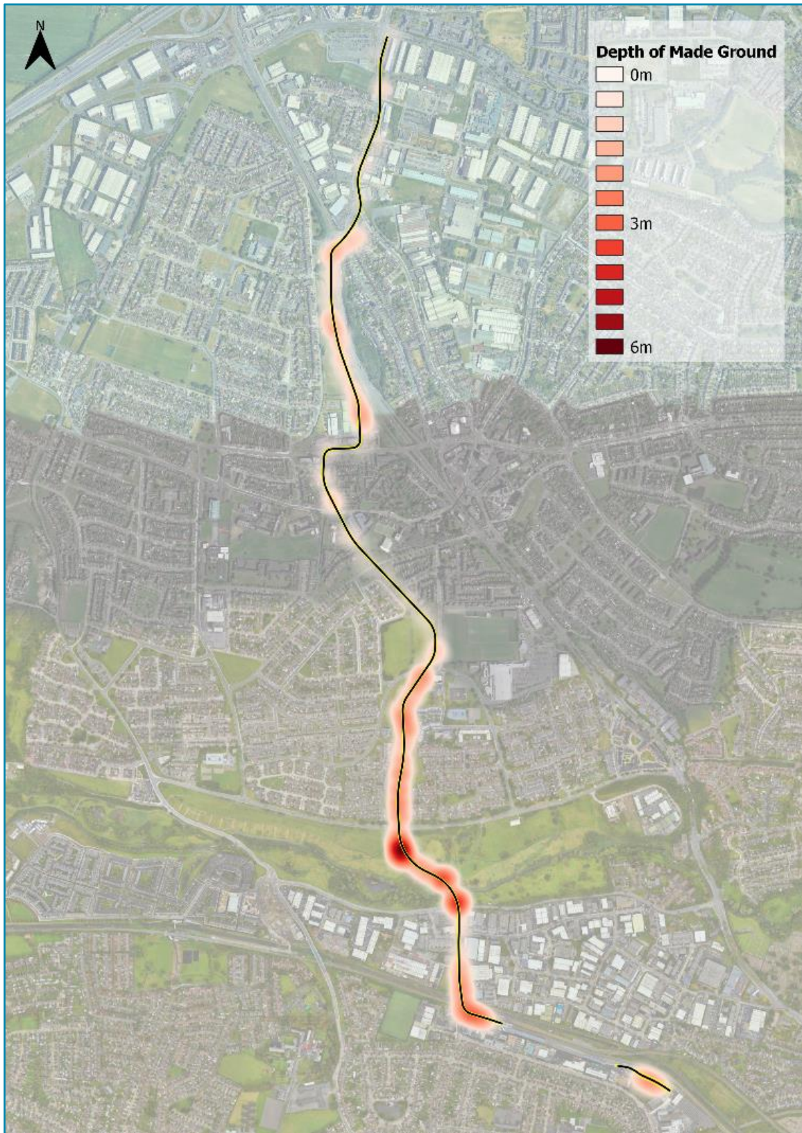
Figure 5-21: Made Ground Deposit Heat Map
